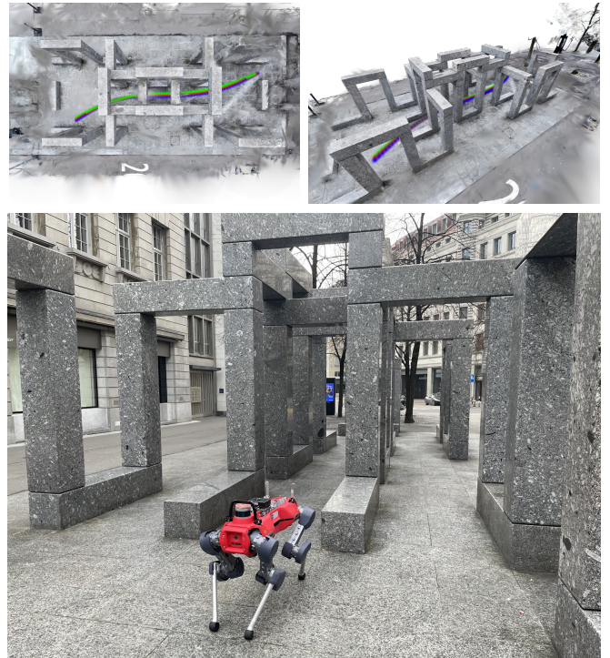
Fig. 4: Trajectories planned for the ANYmal robot through real world obstacles. On the bottom the actual robot can be seen at the site following the trajectories generated by our algorithm FOCI .
